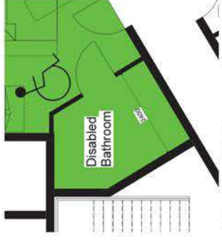
3 Disabled Bathroom without a fixed tracked-hoist system 1 : 50
